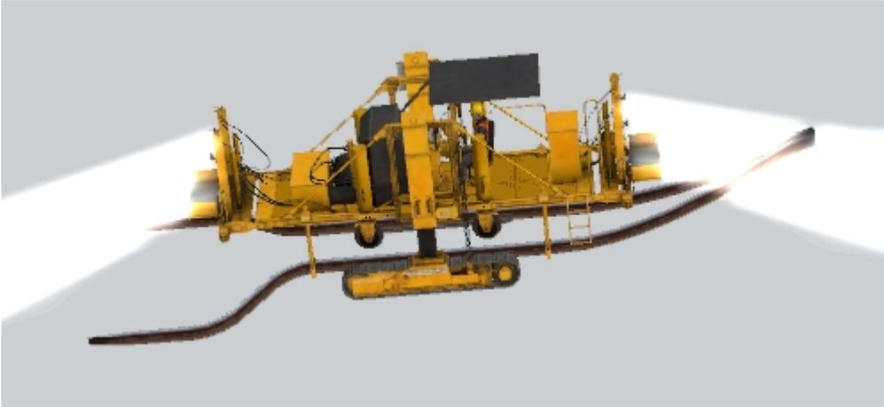
These two machines work together to unload and deposit the rails alongside the embankments in order to prepare the site for the next machine.
