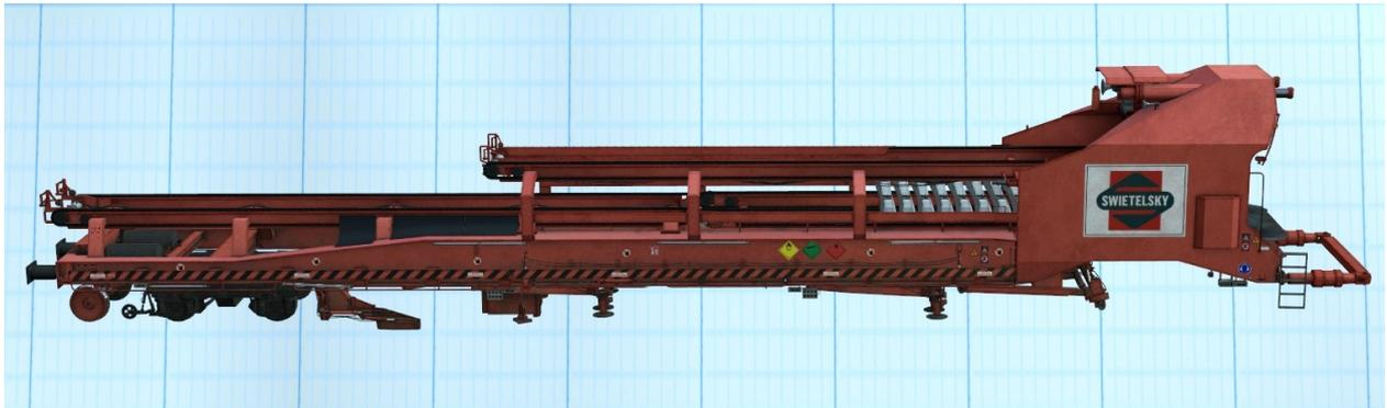
With this set, the old rails and sleepers are first removed and then the new sleepers are laid. The old rails are left alongside the railway.
